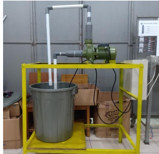
Gambar 6. Water level control berbasis sonoff smart switch Sumber : Dokumen pribadi
