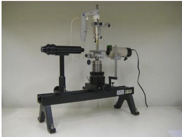
Gambar 5. Drop sensile Goniometer
