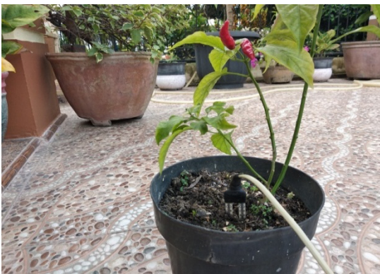
Gambar 14. Pengujian sensor Soil Moisture.
