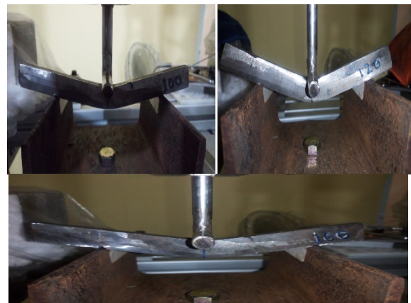
Gambar 5. Proses Uji Bending Spesimen (a) 100 A (b) 120 A dan (c) 140 A
