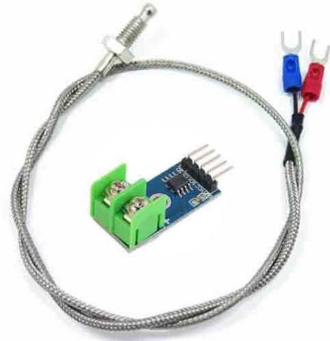
Figure 3. Thermocouple Type-K temperature sensor with MAX6675 module.
