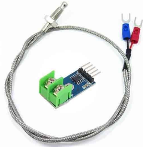
Figure 3. Thermocouple Type-K temperature sensor with MAX6675 module.
